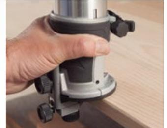
Realization of chamfers or moldings.
